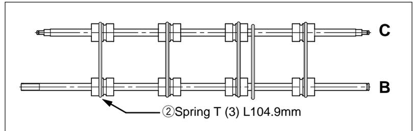
3) Attaching the spring between C, D and E.
