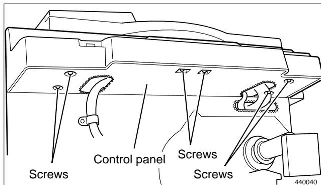
3) Remove the control panel by pulling up.
