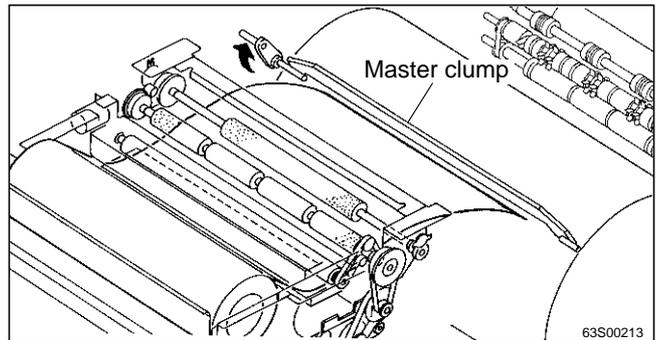
After the master clump is closed and clump the master tip end, the drum rotates to roll up the master.
