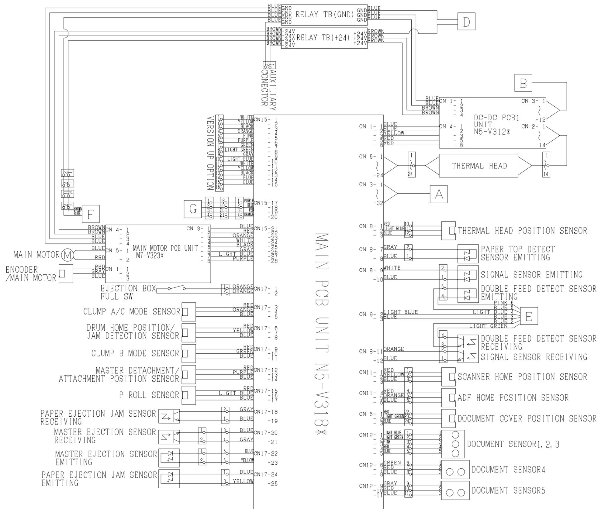
Overall Wiring Layout 1 ( Main PCB ) 2/2
