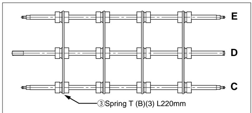
4) Attaching the spring between D, E and F.
