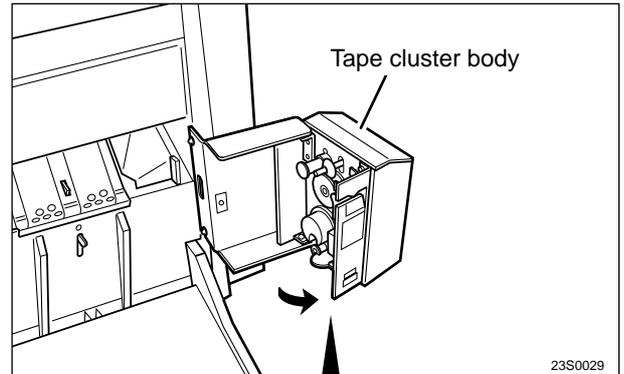
② Install the new tape. Make sure it will wind off in the correct direction.
