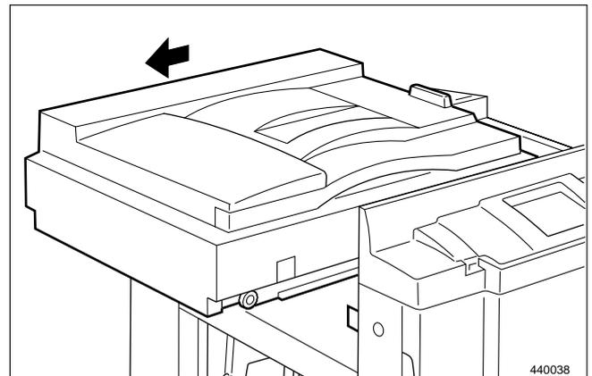
7) Remove the 4 screws, and take out the board cover sliding in the direction of an arrow.
