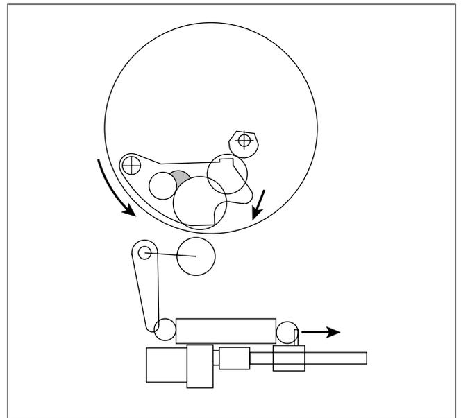
The cam turns a half-revolution, so that the ink roller is pressed against the drum inner surface. Then the drum rotates.
