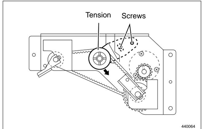
3) Remove the screw to remove the angle.
