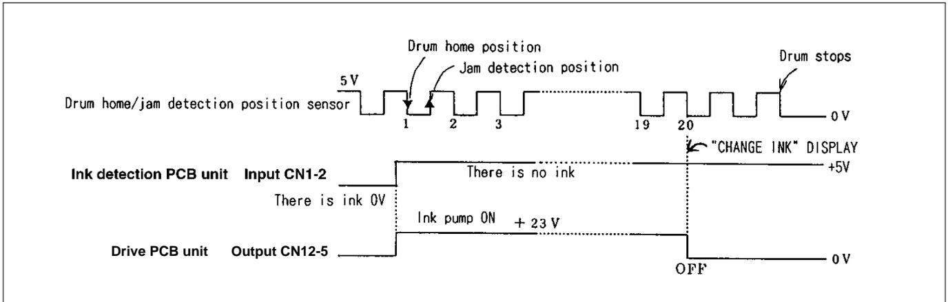
\*The drum rotates until **"CHANGE INK"** is displayed after **HIGH** is output from the ink detection PCB unit during printing. The number of drum rotations varies depending on the printing speed as follows:-
