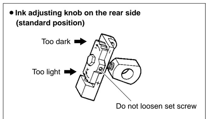
**IMPORTANT :** There are 7 settings, standard and  $\pm 3$  settings to adjust the printing darkness. Print more than ten sheets every time the printing darkness is switched by one setting until the most desirable printing darkness is obtained. Repeat the above procedures until the most desirable printing darkness is obtained.
