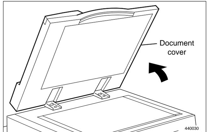
2) Remove the 2 screws shown. Slide the document cover back 1cm, and then pull it up to remove it.
