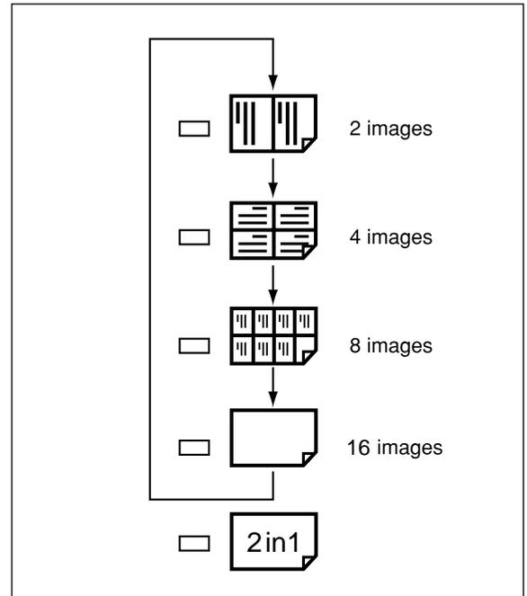
When the ADF is connected, the multiple printing selection key can also be used to select the 2 in 1 Layout Mode, as shown below.
