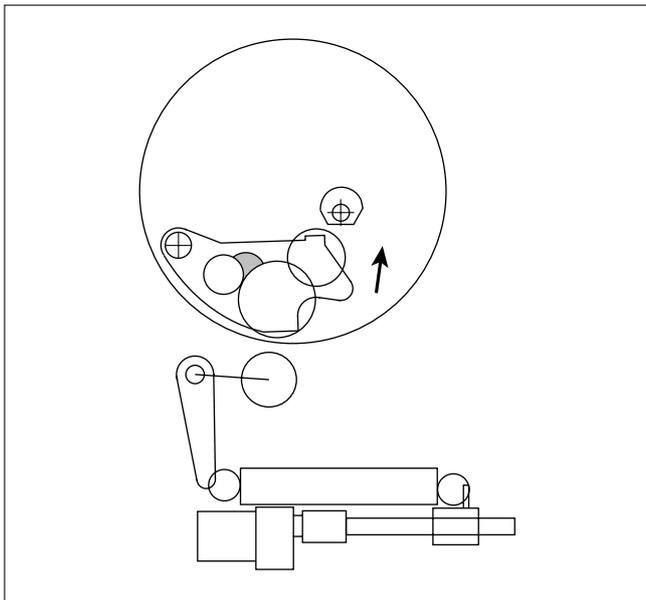
The cam turns a half-revolution, so that the ink roller moves out of contact with the drum inner surface.
