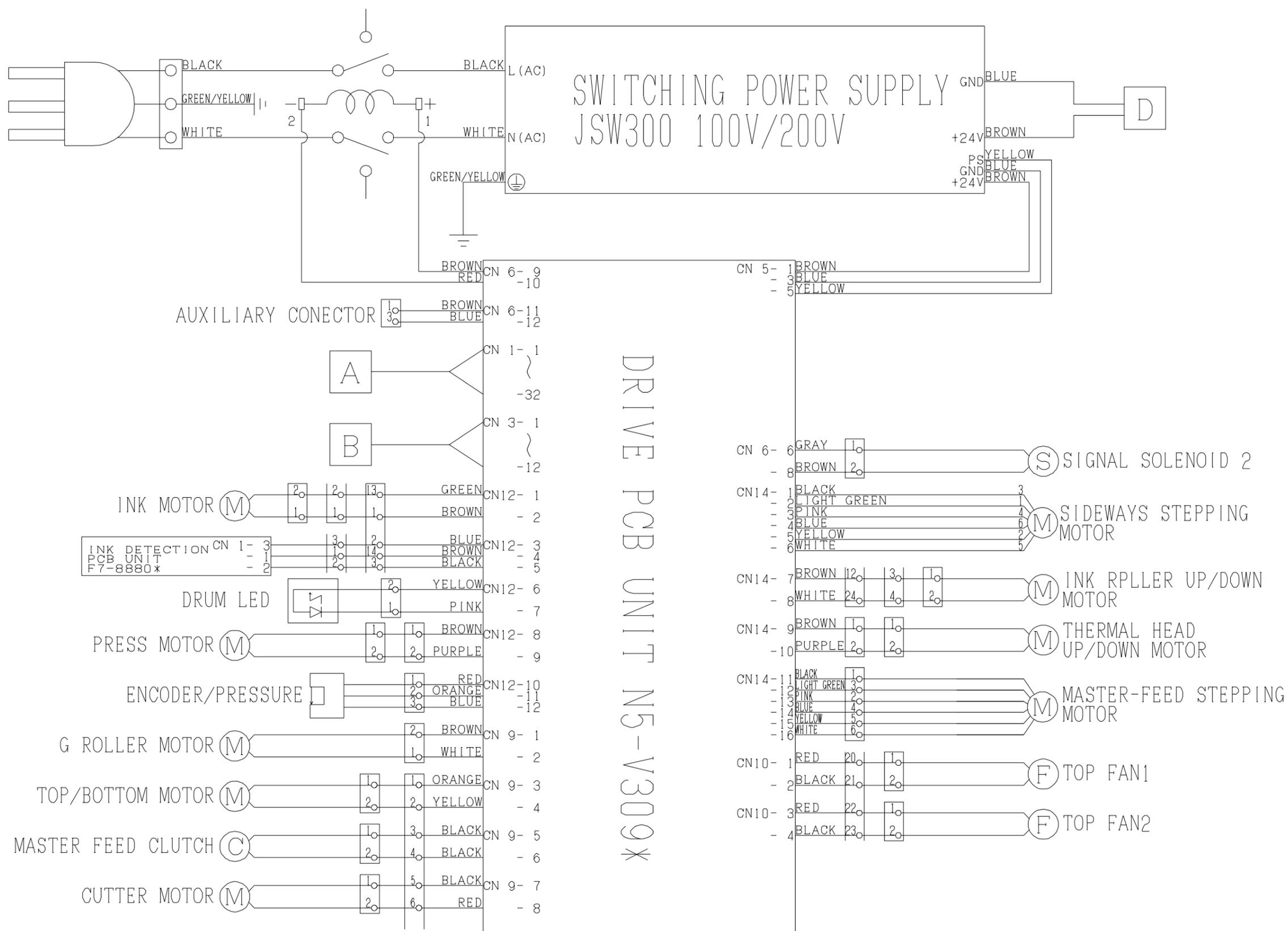
Overall Wiring Layout 2 ( Drive PCB ) 2/2
