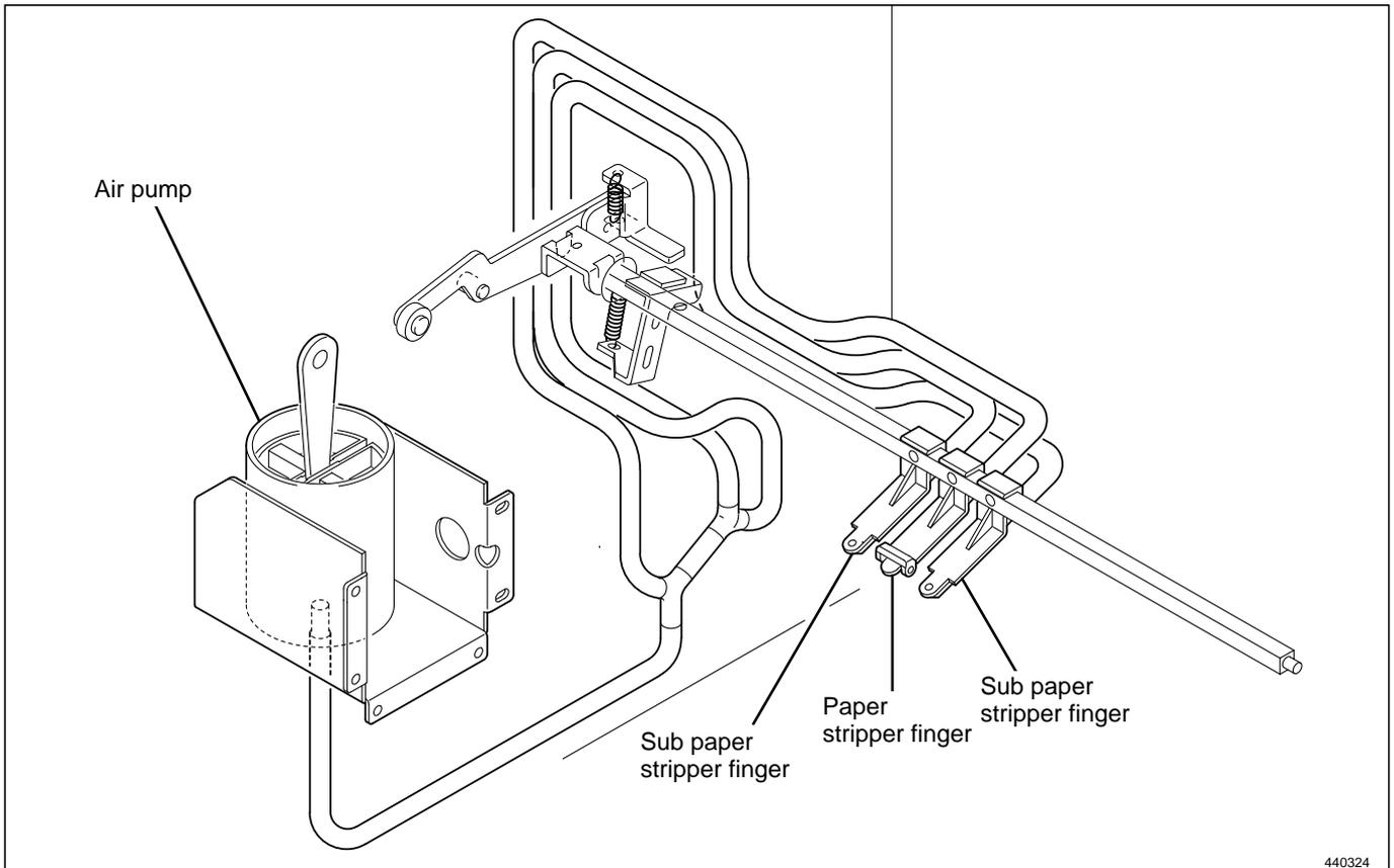
To remove the paper from the drum firmly, the gap between the tip of finger and the drum surface and between the tip of finger and the corner of the master clump are adjusted as follows:-
