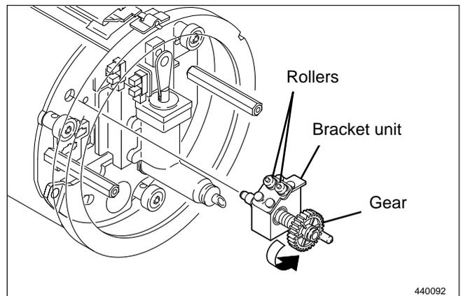
4) Pull out the inner frame (section inside the drum) in the direction of an arrow.
