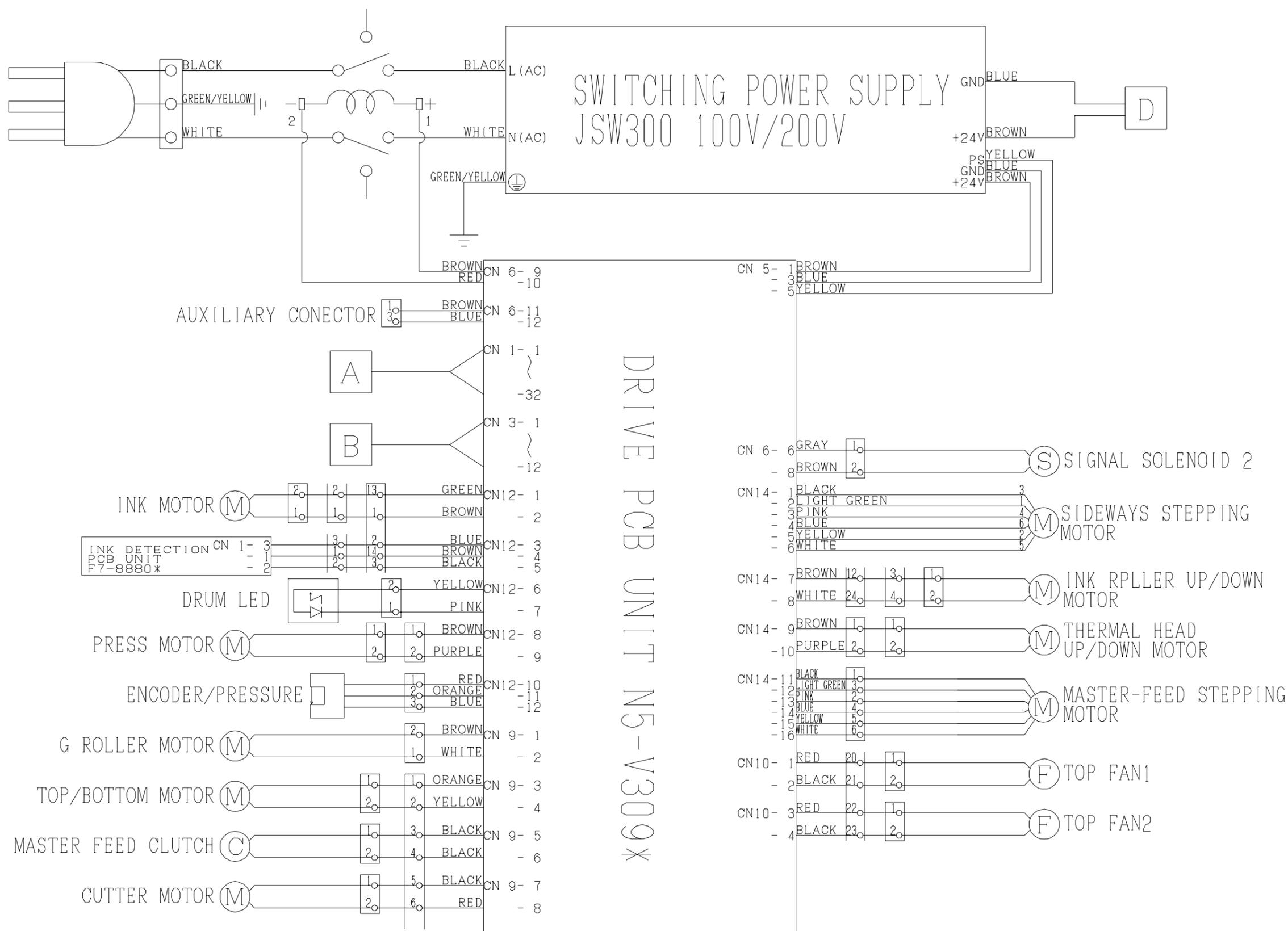
Overall Wiring Layout 2 ( Drive PCB ) 2/2
