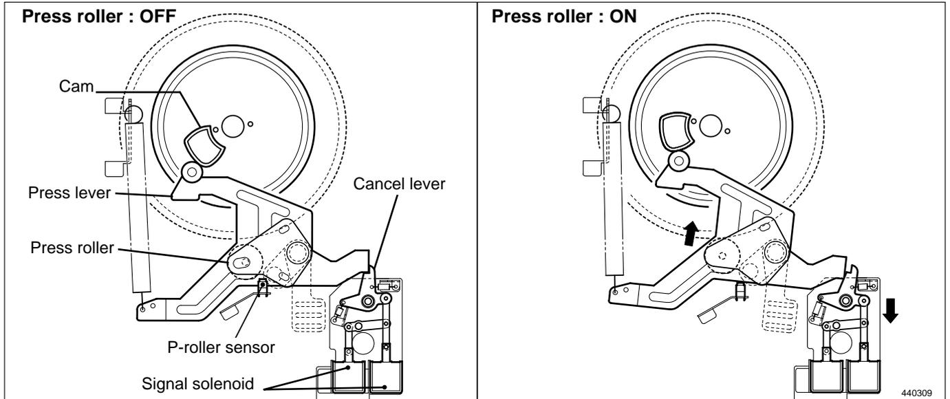
Adjusting the printing area means that the cam curve goes up and down as shown in the figure. The timing of drum ON / OFF varies depending on the cam curve's up and down. The ON position is before the drum hole section, so the printing area is not influenced. (Do not shorten the printing area length as it is influenced.) The OFF position is only changed and the printing area is adjusted.
