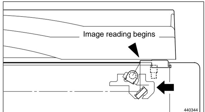
2) When image reading is complete, the lamp goes out, but the optical system decelerates, then stops. Following that, the optical system moves right and returns to the home position.
