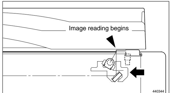
2) The optical system reads the image stopped at home position (PS2). When image reading is complete, it immediately moves to the right and returns to the home position.
