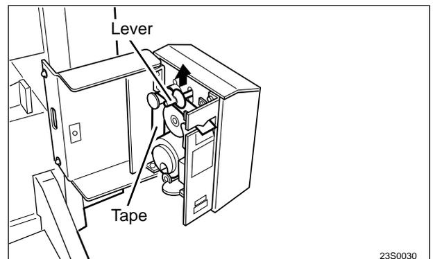
④ Make about 1cm of tape protrude out of the slot.
