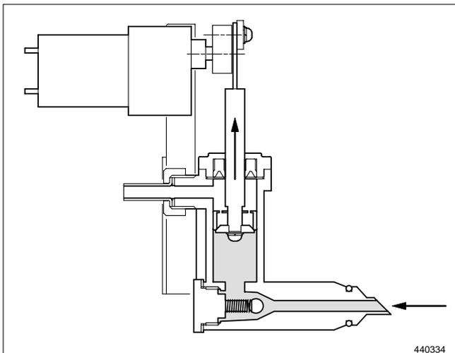
When the piston moves up, it draws ink from the ink pack into the pump.
