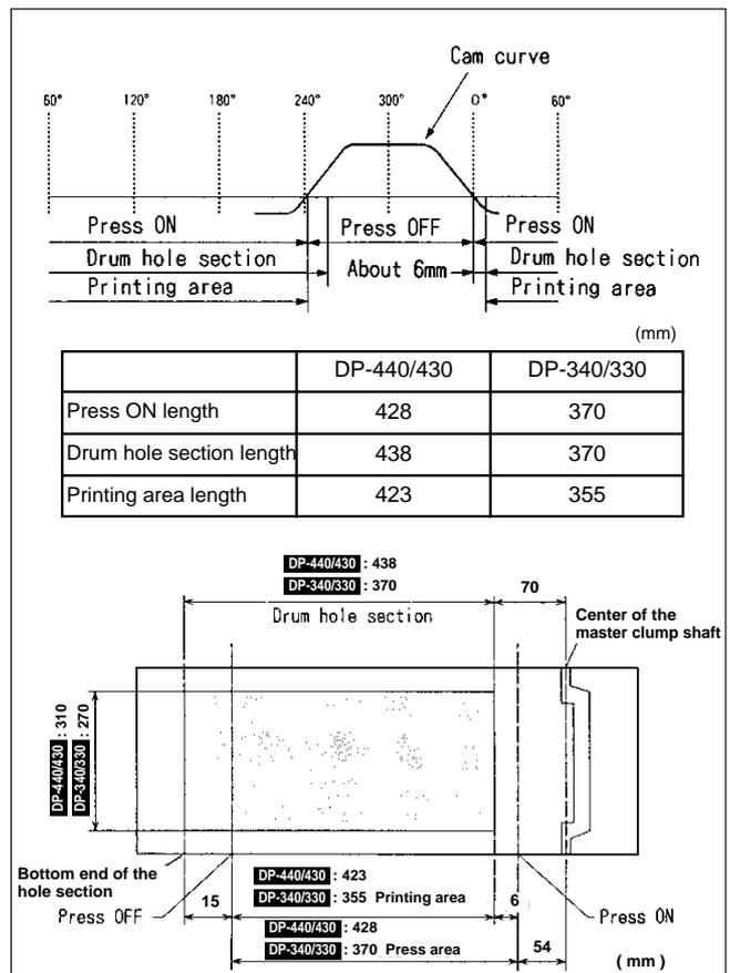
The press roller is ON (the press roller is pressed to the drum) or OFF by operating the press lever up and down with the cam inside the drum gear.
