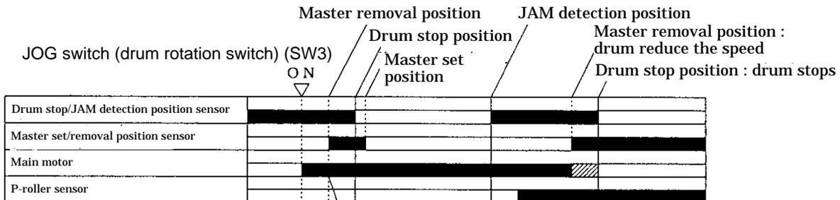
When the P-roller sensor is in the photopassing state (P-roller ON), the drum does not reduce the speed at the master removal position.
