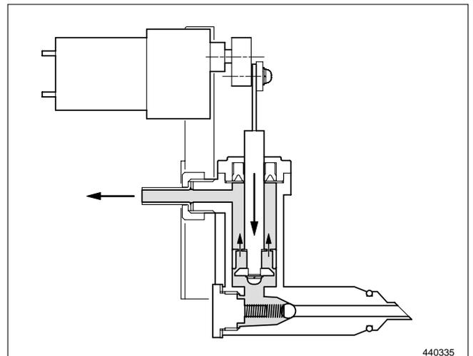
When the piston moves down, the pump releases ink.
