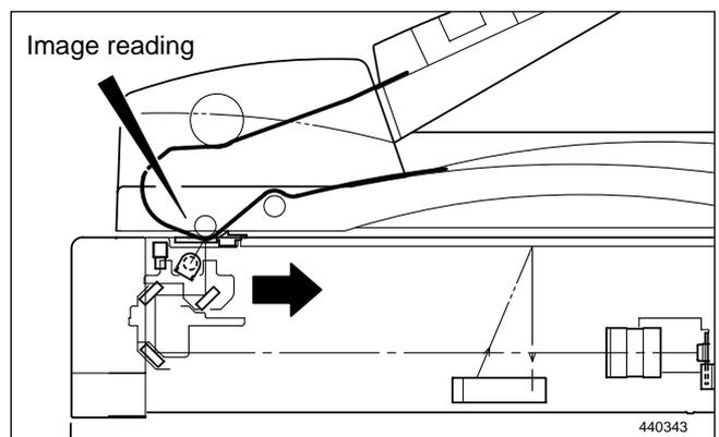
3) After it returns, the optical system is then on standby for the printing process.
