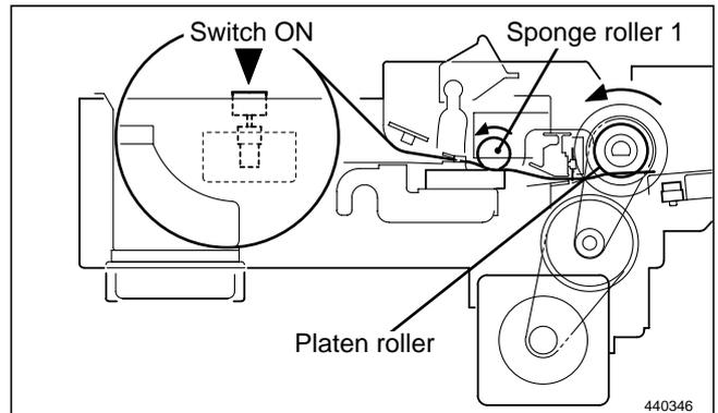
When the master lead edge sensor is interrupted, the master is fed a few steps and stopped. If the master lead edge does not reach the master lead edge sensor, "MASTER SETTING ERROR" is displayed.
