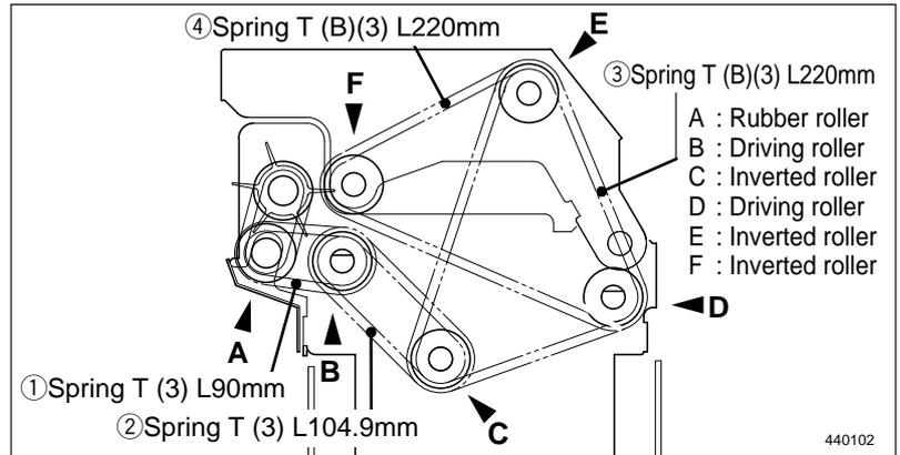
1) Attaching the spring between A and B.
