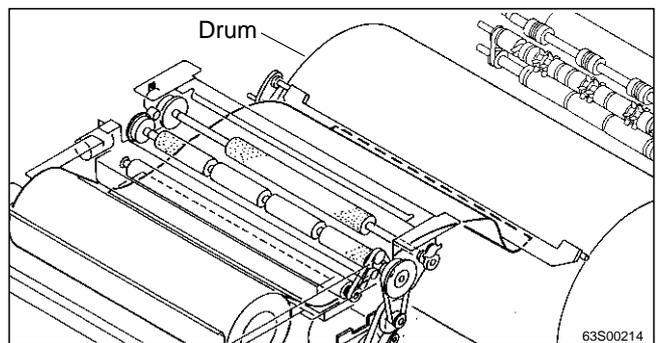
\*Check the length of the master and drum rotation angle to control the drum rotation.
