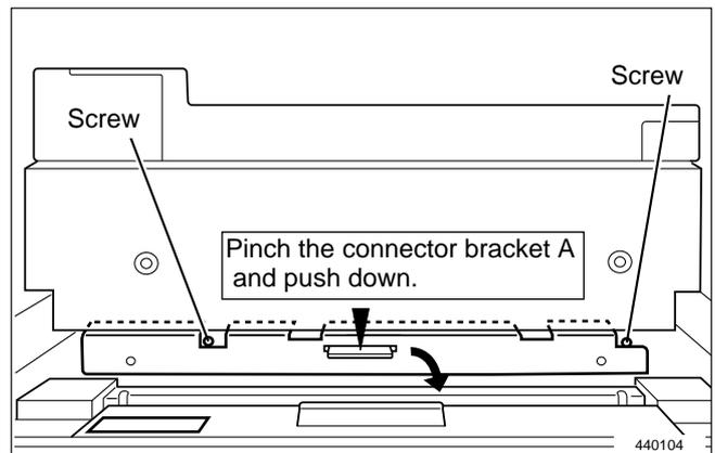
5) Remove the 2 screws indicated, then remove the side cover L.
