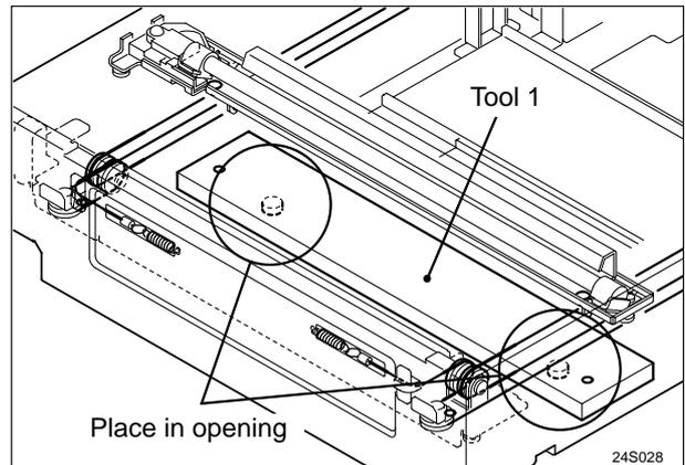
2) Turn the timing pulley and move Slider A so that the Slider A positioning openings are aligned with the Slider A attachment tool 1 positioning openings.
